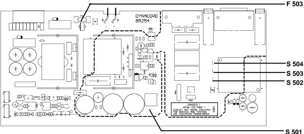
Fig. 3 PCB 85254 Location of the wire jumpers S501 - S504 for altering mains voltage and position of the output fuse F503
